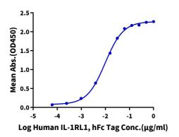
Immobilized Human IL-33, No Tag at  $5\mu g/ml$  (100 $\mu$ I/well) on the plate. Dose response curve for Human IL-1RL1, hFc Tag with the EC50 of 9.8ng/ml determined by ELISA (QC Test).
